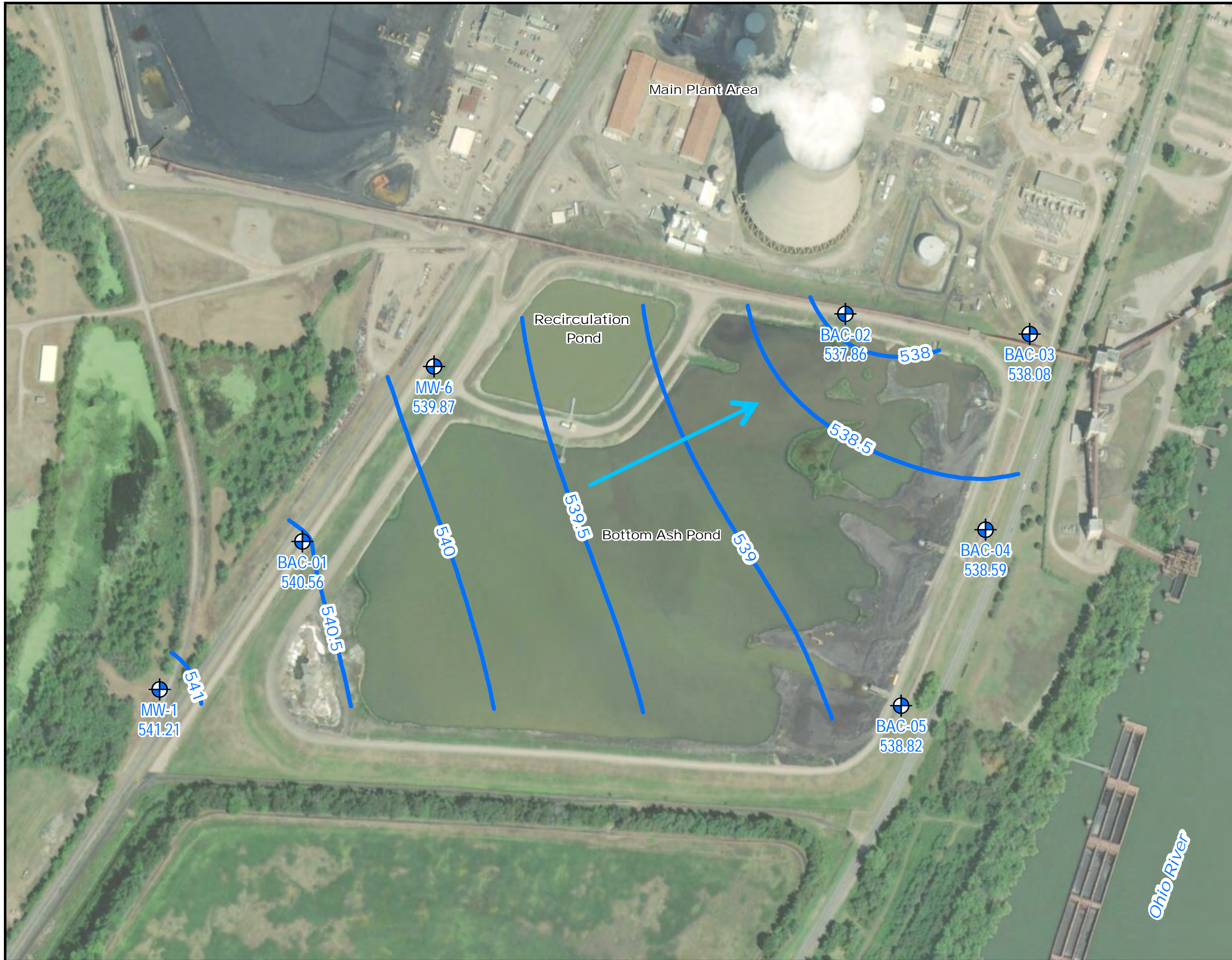
Figure 3-5: March 2017 Groundwater Elevations and Flow Direction Bottom Ash Complex Alternate Source Demonstration Gavin Generating Station Cheshire, Ohio
