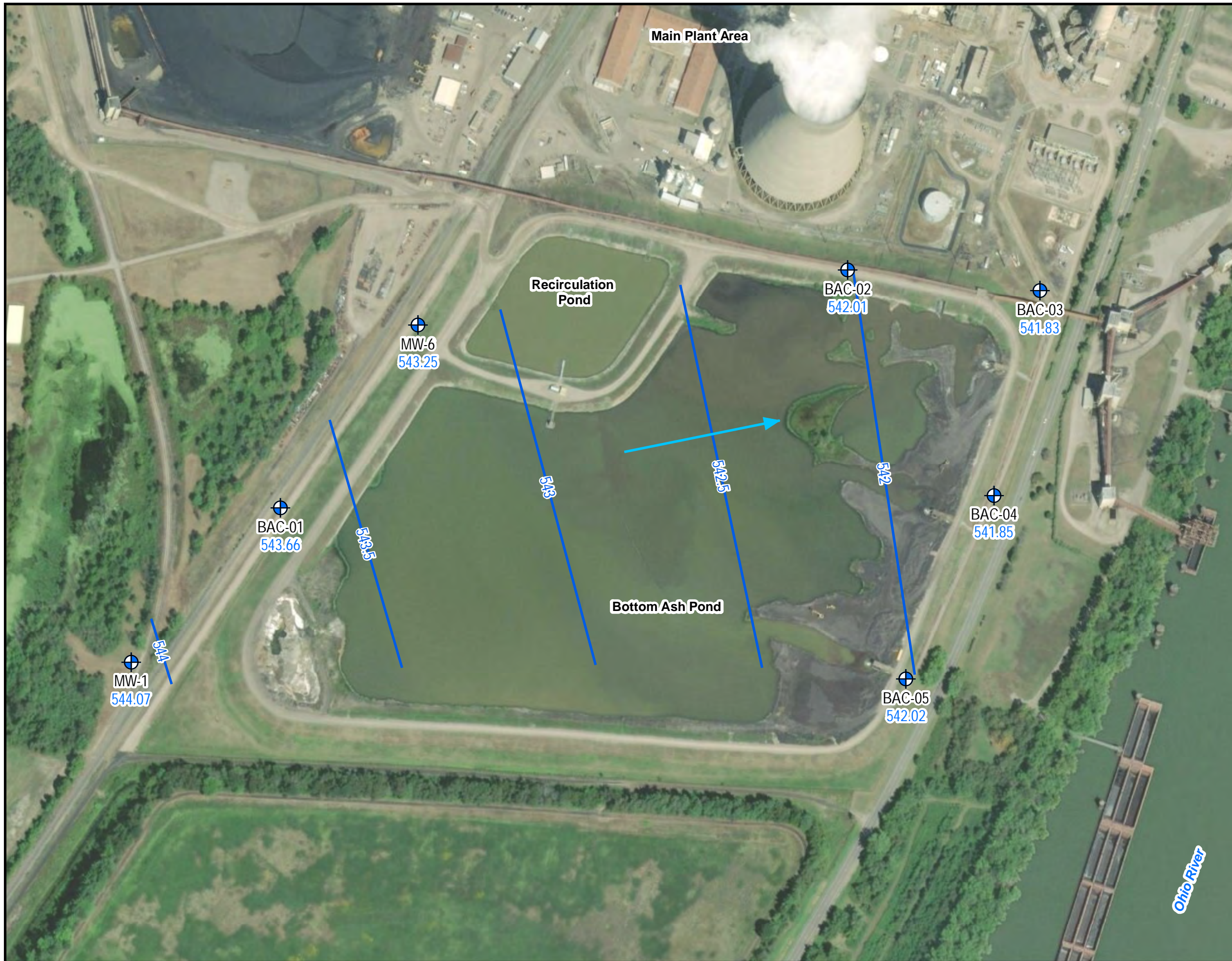
Figure 3-1: May 2018 Groundwater Flow Direction Bottom Ash Complex Annual Groundwater Monitoring and Corrective Action Report Gavin Power Plant Cheshire, Ohio
