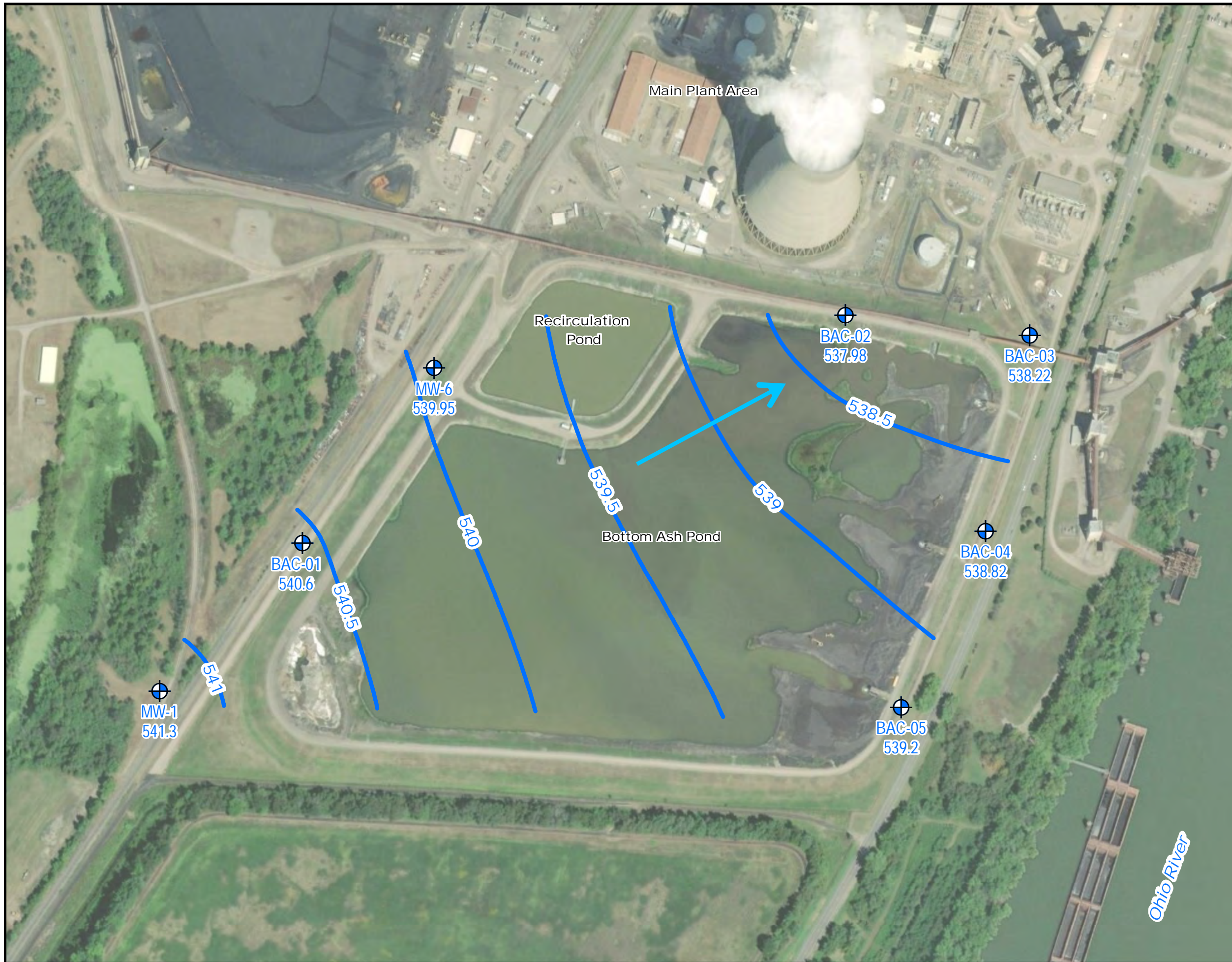
Figure 3-7: June 2017 Groundwater Elevations and Flow Direction Bottom Ash Complex Alternate Source Demonstration Gavin Generating Station Cheshire, Ohio
