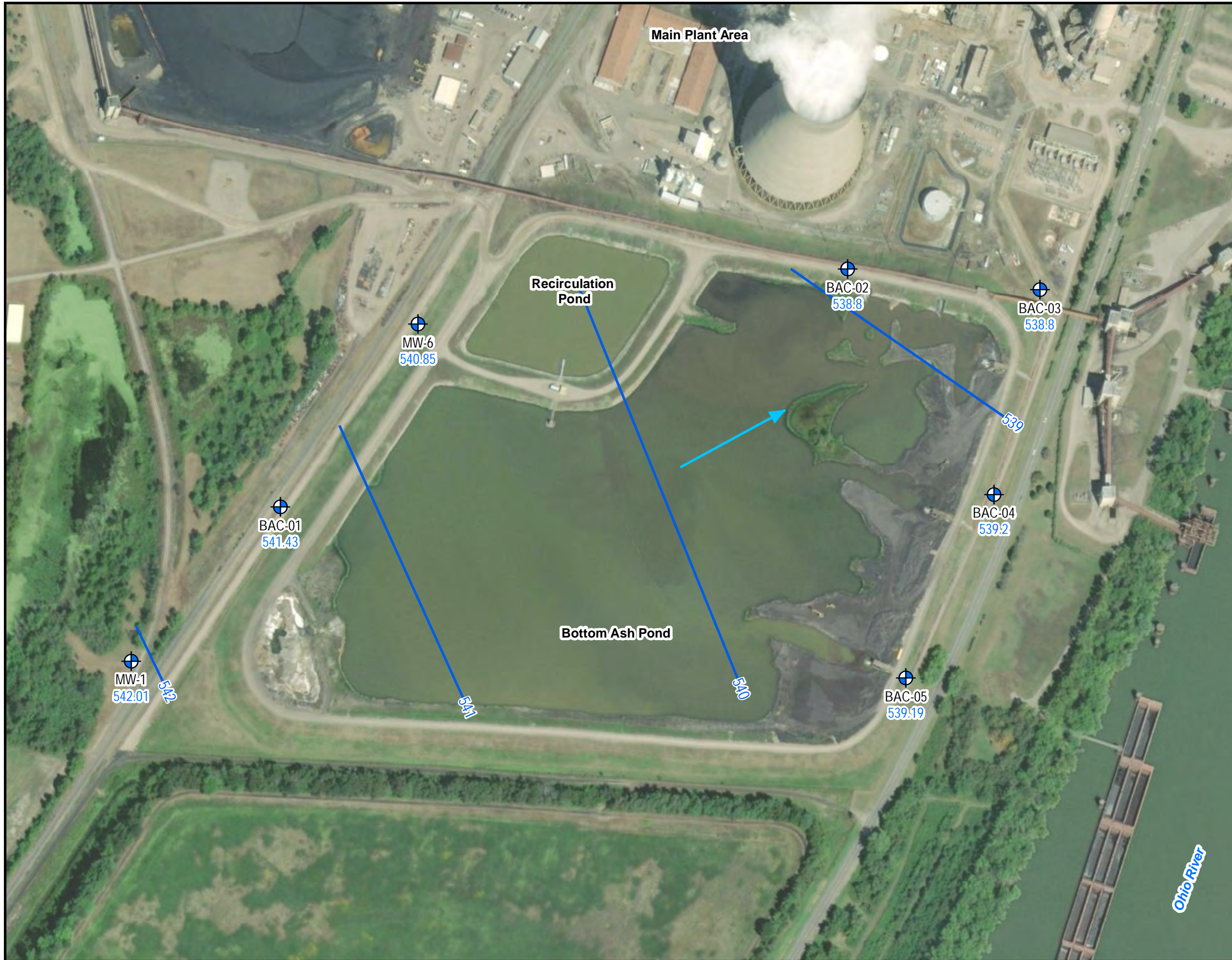
Figure 3-2: September 2018 Ground-water Flow Direction Bottom Ash Complex Annual Groundwater Monitoring and Corrective Action Report Gavin Power Plant Cheshire, Ohio
