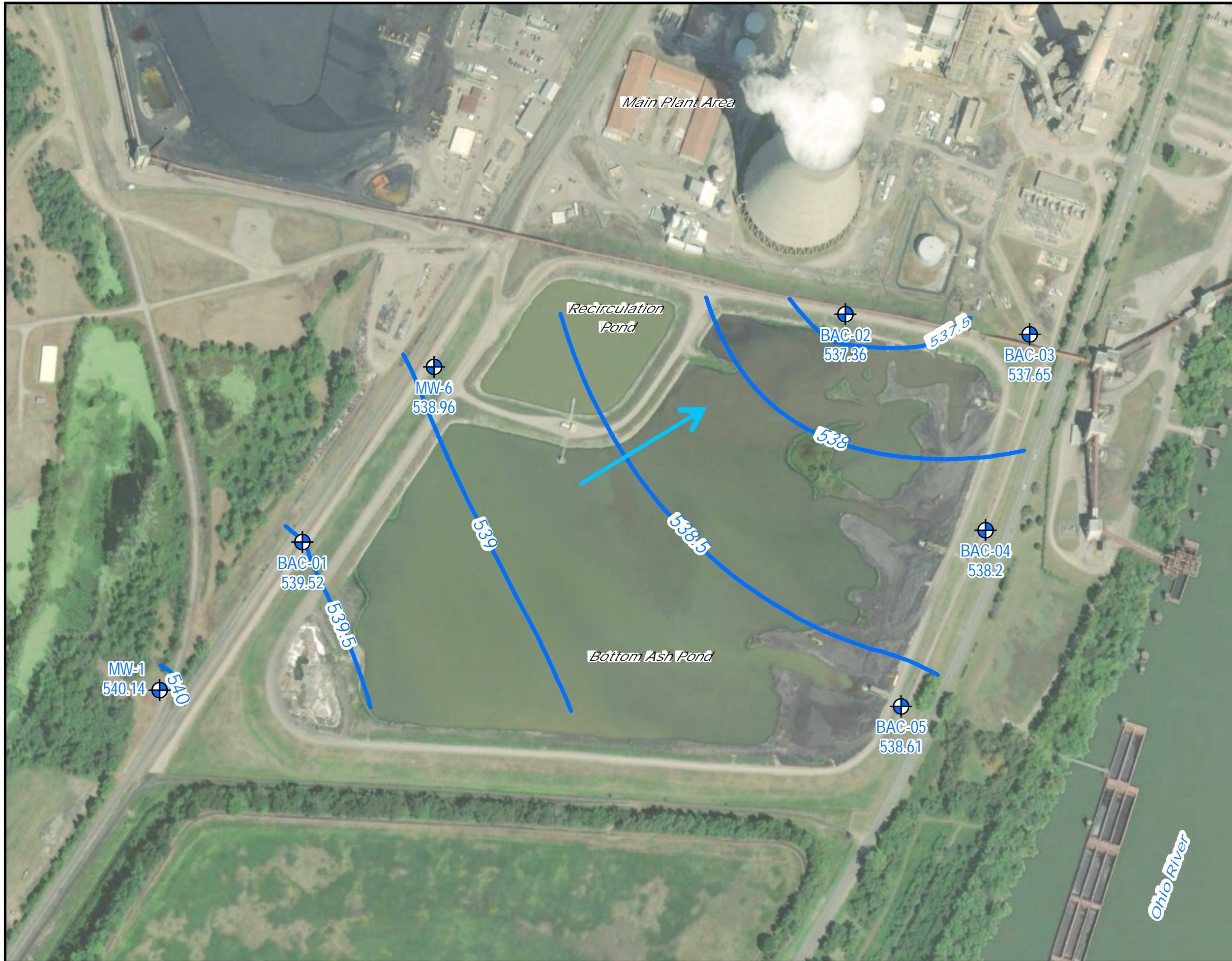
Figure 3-2: October 2016 Groundwater Elevations and Flow Direction Bottom Ash Complex Alternate Source Demonstration Gavin Generating Station Cheshire, Ohio
