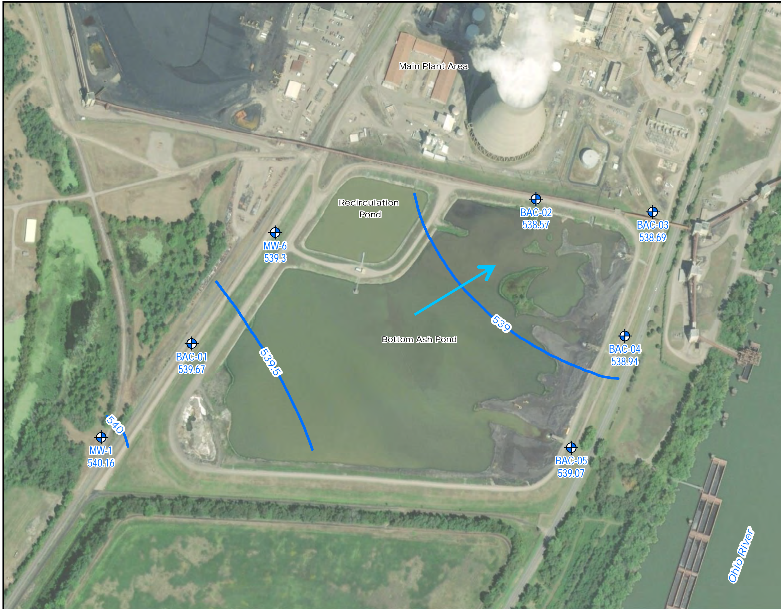
Figure 3-3: November 2016 Groundwater Elevations and Flow Direction Bottom Ash Complex Alternate Source Demonstration Gavin Generating Station Cheshire, Ohio
