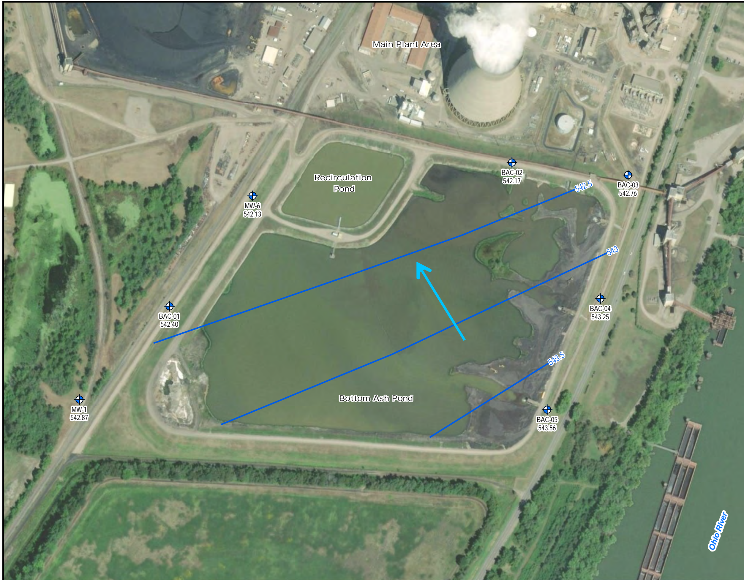
Figure 3-4: February 2017 Groundwater Elevations and Flow Direction Bottom Ash Complex Alternate Source Demonstration Gavin Generating Station Cheshire, Ohio
