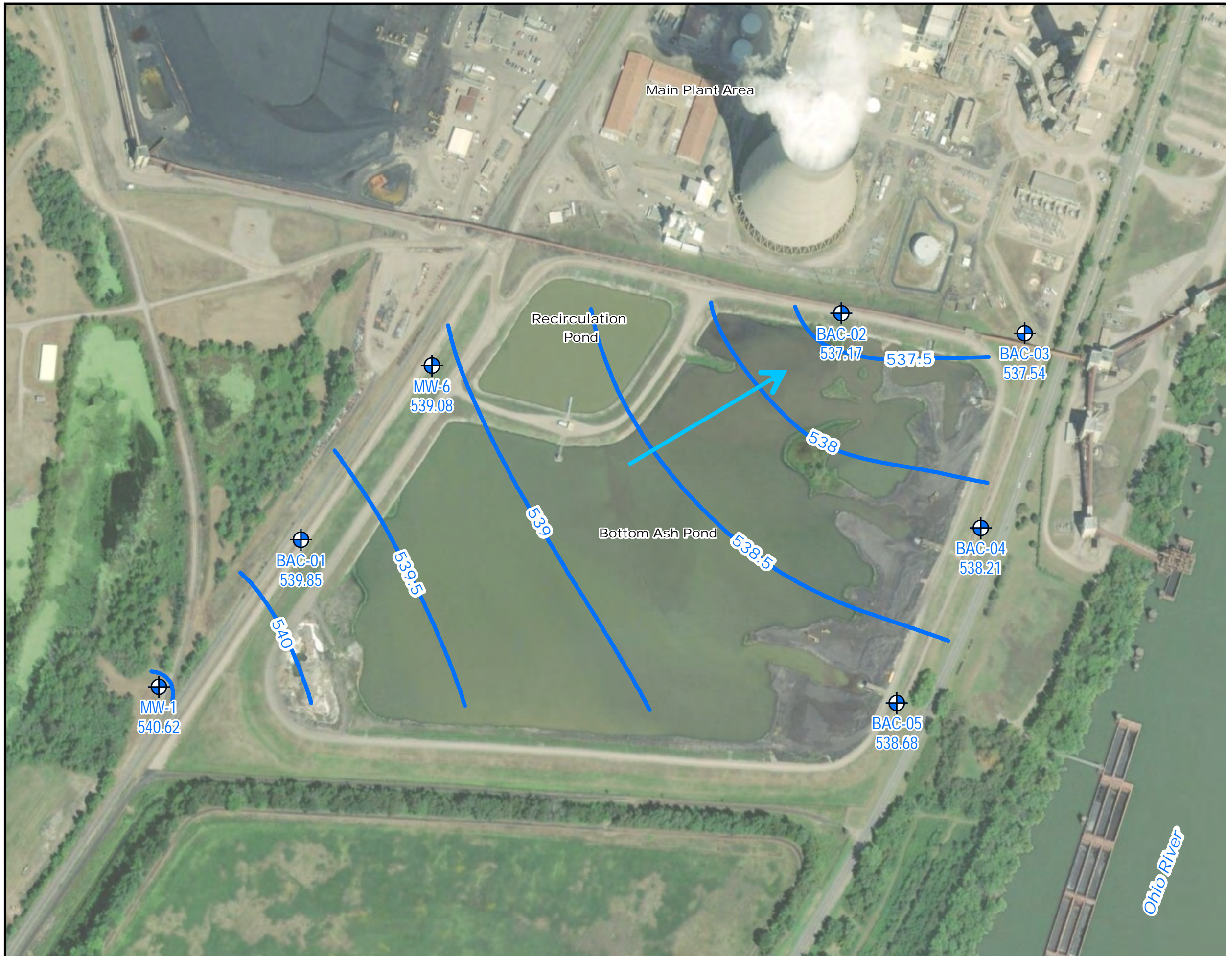
Figure 3-8: July 2017 Groundwater Elevations and Flow Direction Bottom Ash Complex Alternate Source Demonstration Gavin Generating Station Cheshire, Ohio
