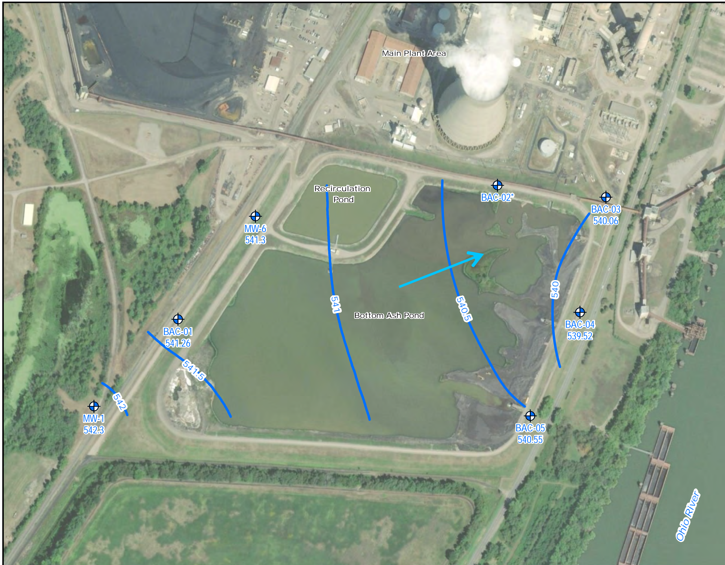
Figure 3-6: May 2017 Groundwater Elevations and Flow Direction Bottom Ash Complex Alternate Source Demonstration Gavin Generating Station Cheshire, Ohio
