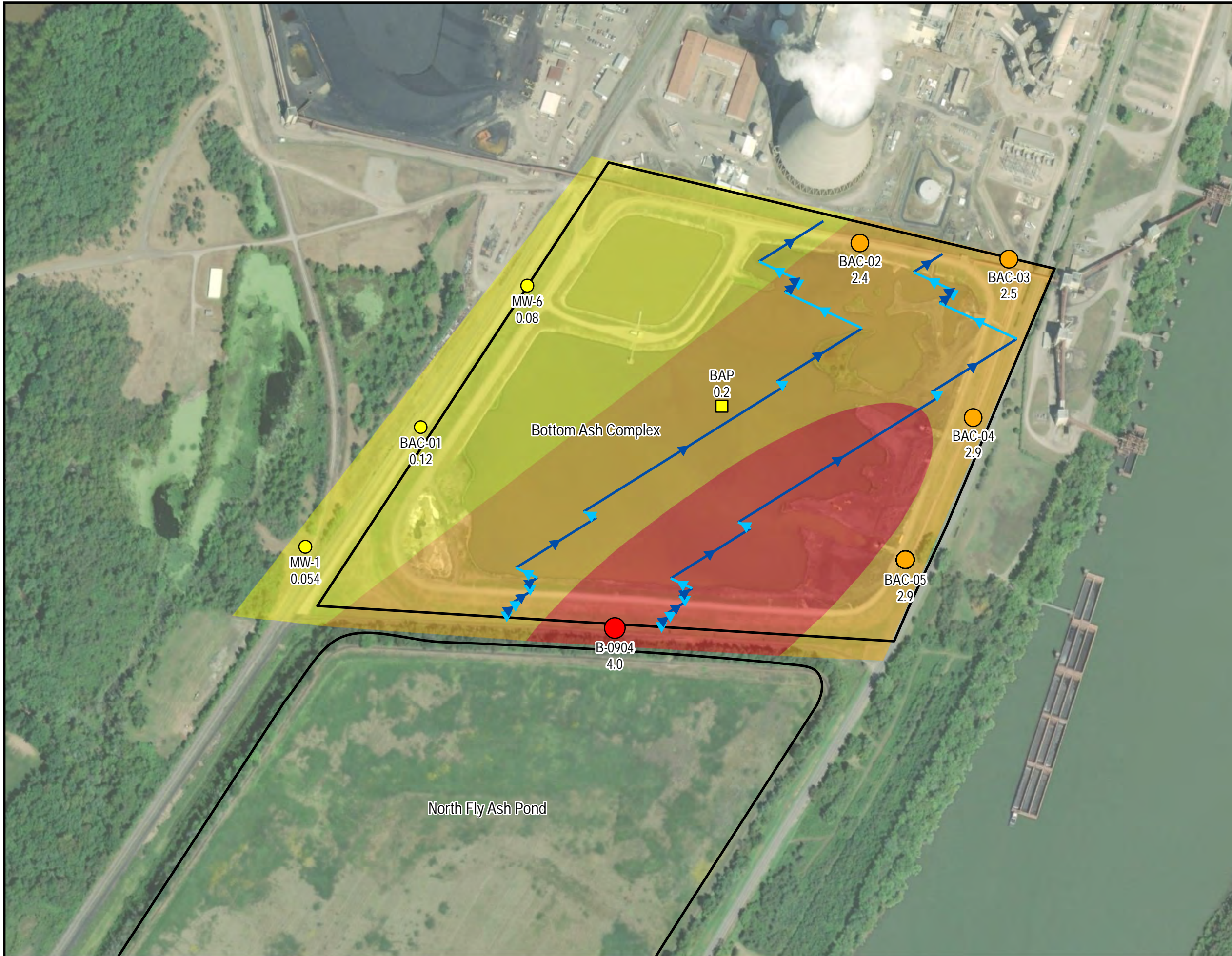
Figure 4-3: Boron Distribution in Groundwater in May 2018 Bottom Ash Complex First Semi-Annual Sampling Event of 2018 Alternate Source Demonstration Gavin Generating Station Cheshire, Ohio
