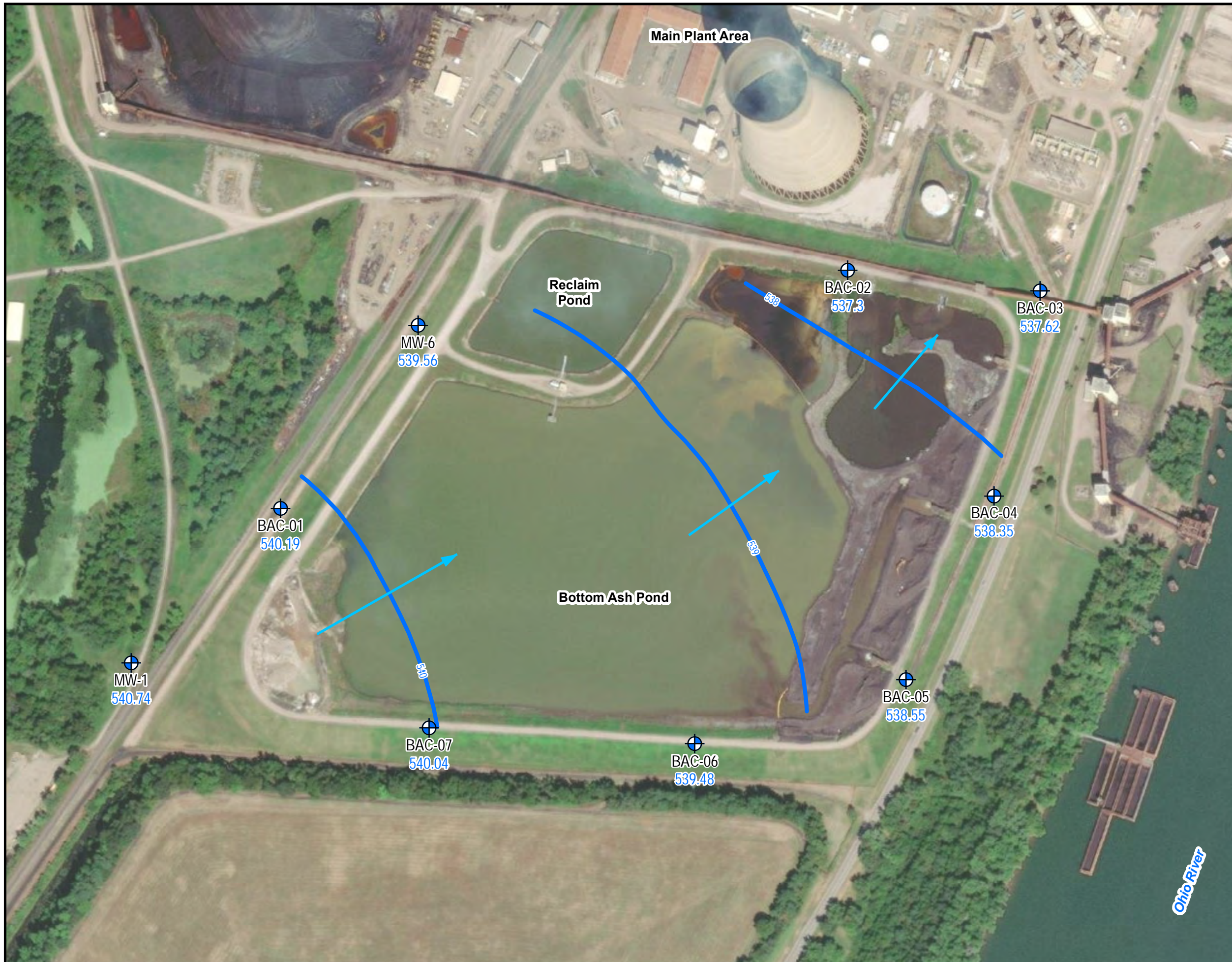
Figure 2-2: Interpreted Groundwater Potentiometric Contour September 2021 Gavin Power, LLC Cheshire, Ohio
