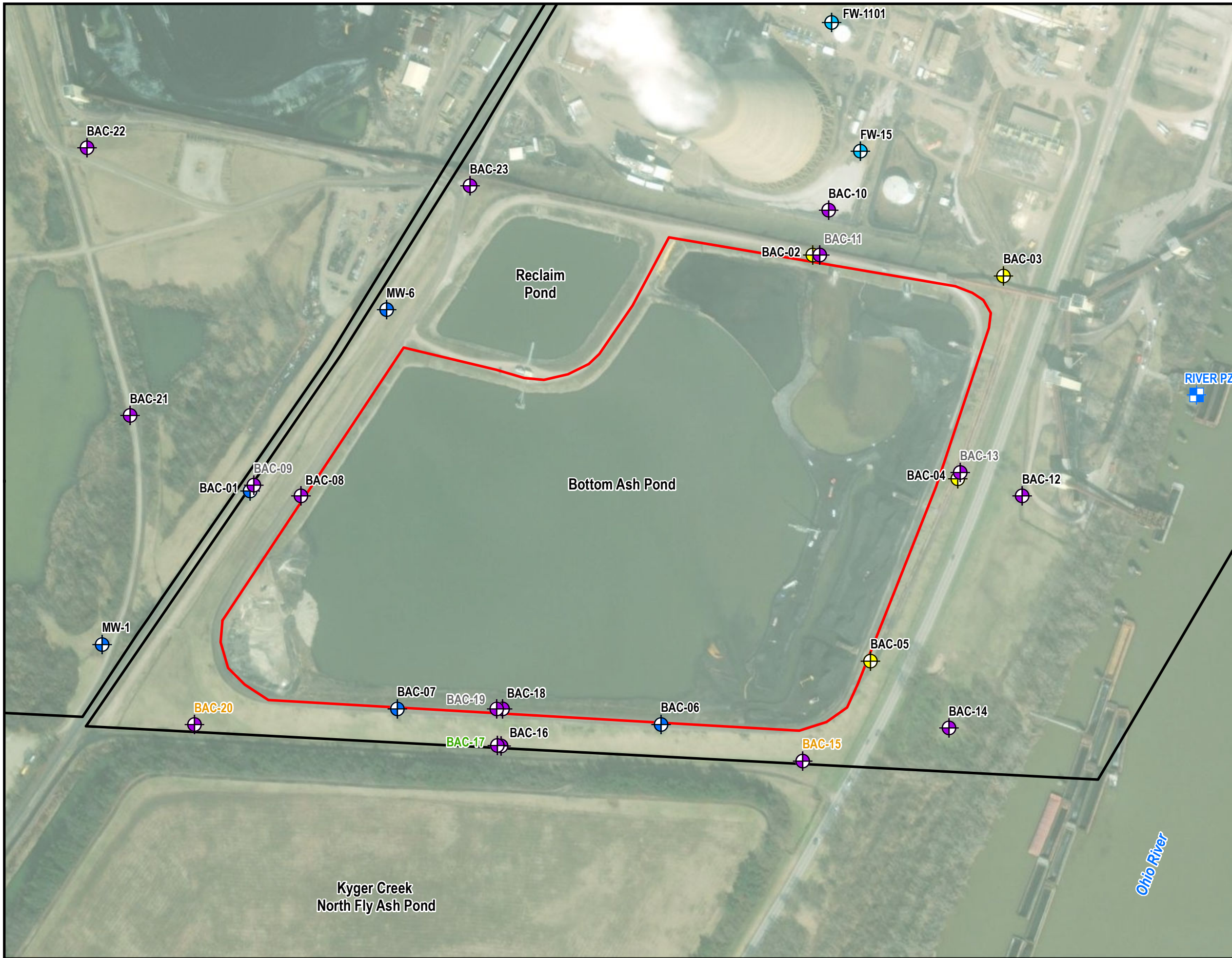
Figure 3-3: Bottom Ash Pond Monitoring Well Network Gavin Generating Station Cheshire, Ohio
