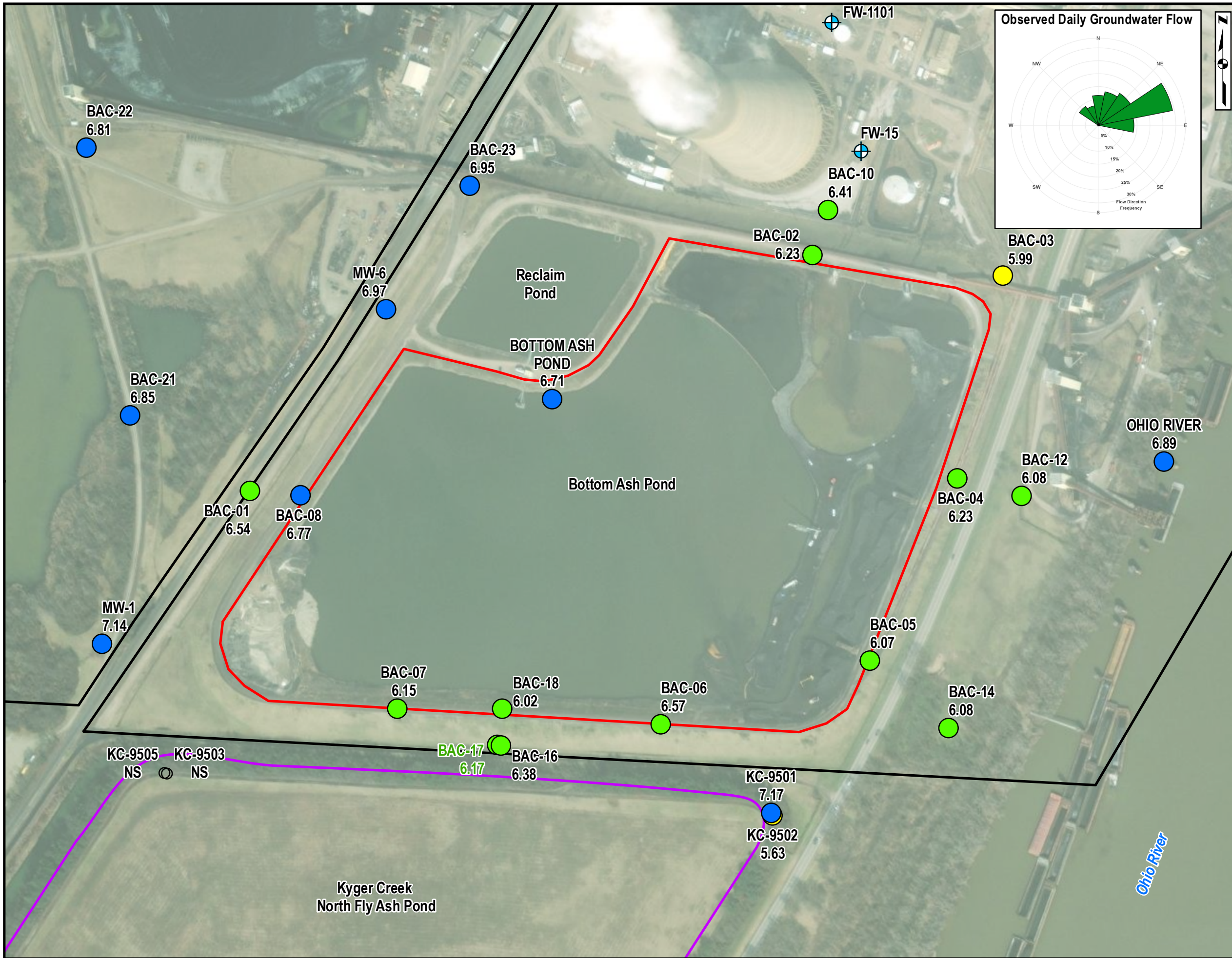
Figure 4-7: pH Distribution in Groundwater (Map View) Gavin Generating Station Cheshire, Ohio
