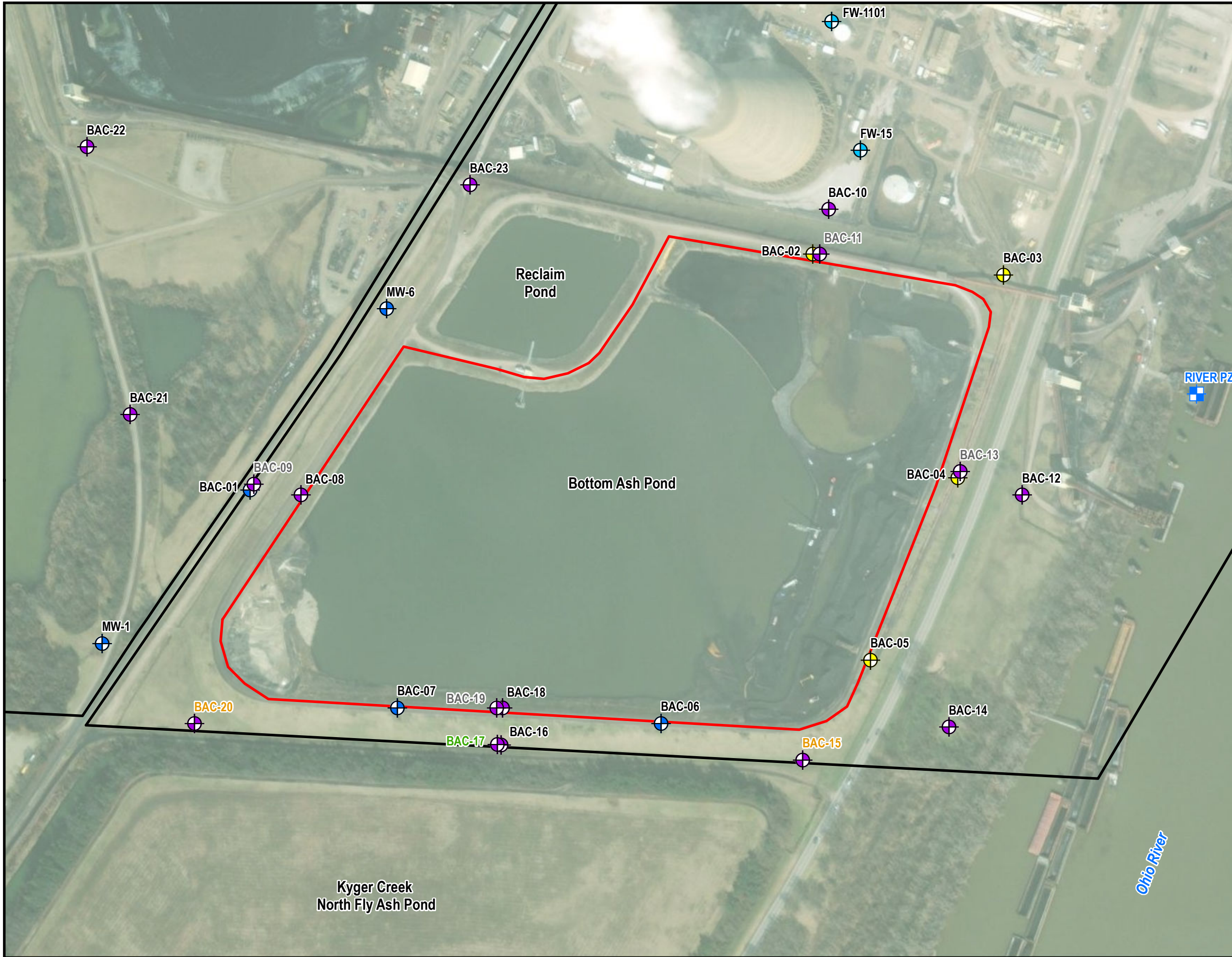
Figure 1-3: Bottom Ash Pond Monitoring Well Network Gavin Generating Station Cheshire, Ohio
